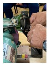
Next up was the Bowl Gouge also to 45° using a jig. The tip here was to over rotate whilst grinding to ensure that the wings of the gouge aren't proud opening up an increased risk of a catch.
