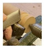
When using a Skew, be gentle with both your grip and how you rest the tool on the wood.
