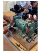
gouge is ground more and a dip occurs. Check by eye and rectify as necessary.
