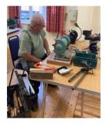
Nick began with his Spindle Roughing Gouge using a ruby wheel/120G grinding to 45°. Top tip here whilst grinding is to pause on the wings of the gouge before returning to ensure an even amount of time and grind across the width of the tool. Otherwise the middle of the
