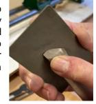
Mick recommends maintaining tool rests with a draw file (in one direction at -45° to perpendicular and then the opposite direction at +45° followed by sand paper) to keep smooth as any nicks in the rest will transfer through the tool on to the wood – "Tool rests should be smooth"
